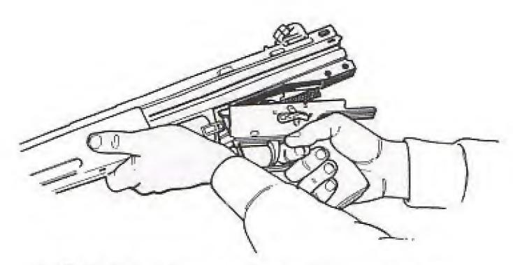
3. Reinstall the trigger group by first inserting the front of the trigger group, then rolling the rear end with the pistol grip into position.
